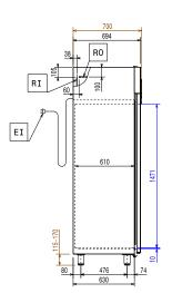
Electrical inlet (power) Refriaerant Inlet Refrigerant Outlet
